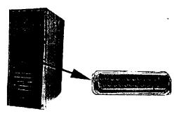
5. If your printer is already connected to the parallel port on the back of your computer, unplug the printer cable and plug it into the connector labeled "To Printer" on the back of the MediaMaster drive.
